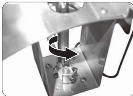
4. Mount the 2mm injector for natural gas.
