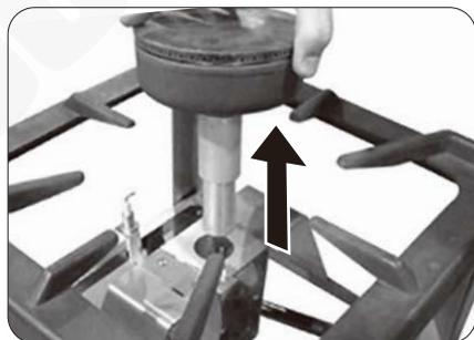
3. Unscrew the 1.15mm injector and save for future use.
